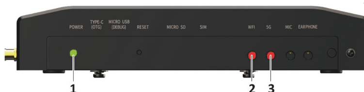
Figure 3-4. Front View Light Location
