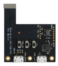
The USB board contains two micro USB and one JTAG interface:
