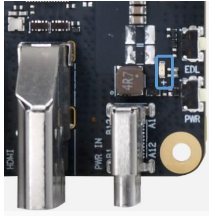
图3-10. 电源指示 LED
