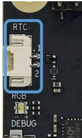
Figure 3-7. RTC Battery Connector
